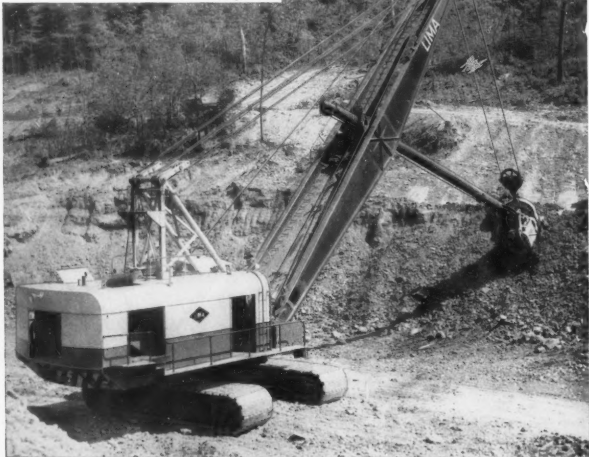
6 or 8-yd. Lima Type 2400, shown stripping coal in Pennsylvania, also available with special 10-yd. coal loading dipper.
